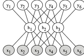
Fig. 2. The graphical model corresponding to the application of a CFOE to a sequence. The bottom row of shaded nodes corresponds to the observations, which are always observed. The top row are the labels, which are observed during training but latent during testing. The middle row are the variables corresponding to the features; these are always latent. In this CFOE,  $N = 3$ .
